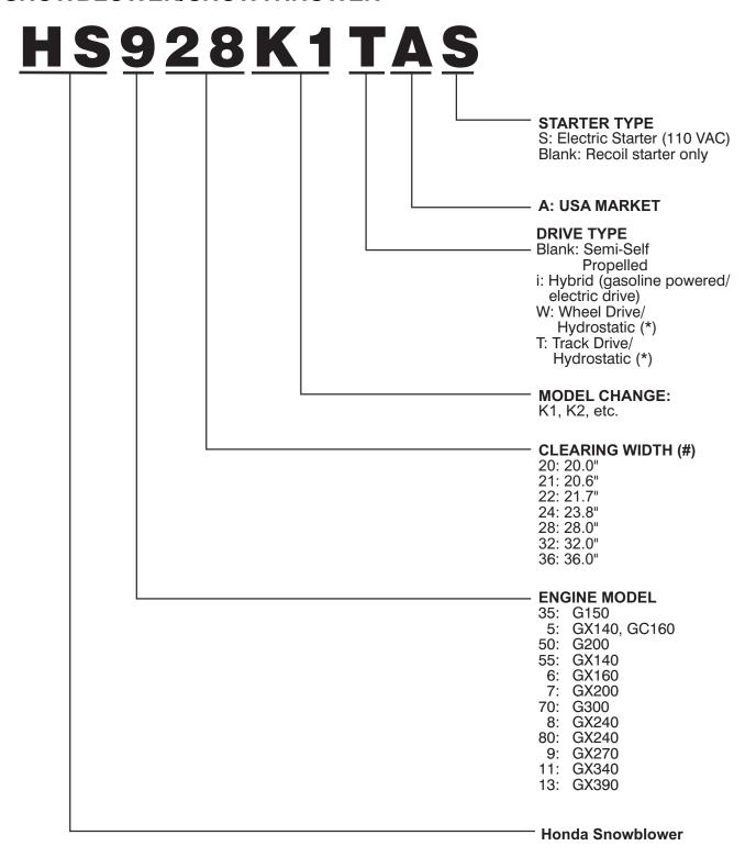
(\*) Early wheel and track drive models were gear drive (2 forward, 1 reverse).
